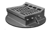
Suitable for 24" curb and gutter, split frame facilitates forming and eliminates boxing out. When paving roadway, simply place small section of frame against the form on the pavement side at catch basin location. After forms are removed, attach large frame section and curb box using bolts provided, and pour curb and gutter section. If curb and gutter are installed first, reverse the procedure.
